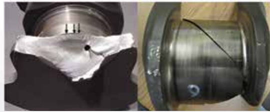
Bending fatigue failure
