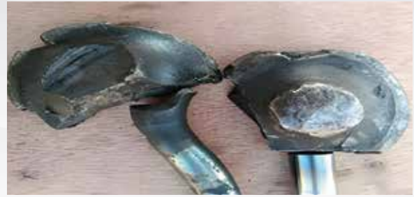
Sticking valve from carbon deposits
